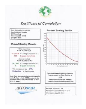
Example of results: computer printout from one of the five separate duct systems sealed with Aeroseal.
